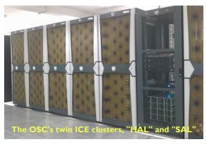
SAL is an Altix ICE cluster from SGI and comprised of 80 nodes, each with two quad core processors (640 cores in total compared to HAL's 528). Each processor is of the new Intel "Nehalem" generation which delivers greatly increased performance over previous Intel offerings by removing the performance bottleneck between the processor and main memory: it is not unknown to see performance double for the same clock speed processor as a result.
