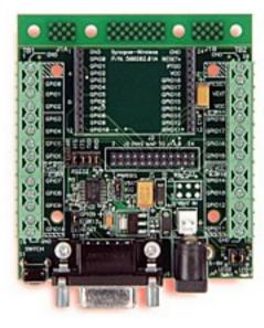
"...IEEE802.15.4 based, auto-forming, multi-hop, instant-on, mesh network stack combined with an embedded Python interpreter for running application code."
