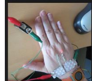
Body Power Tattoo - see red Light emitting Diode is lit up via circuit tracks on the skin
