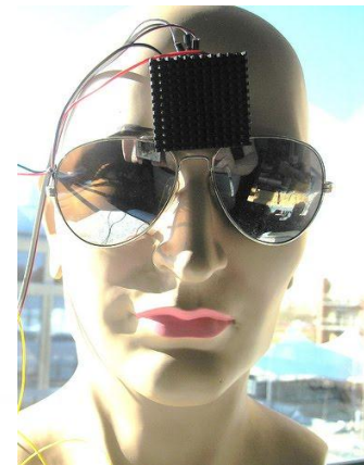
ThrillChip V2 - note heatsink for Peltier chiller
